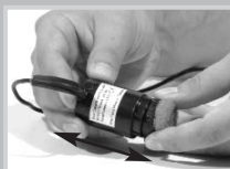
Remove pump base
