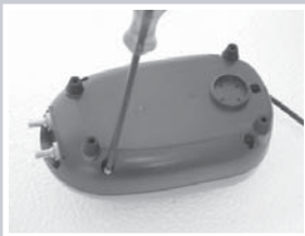
Unscrew on the bottom
